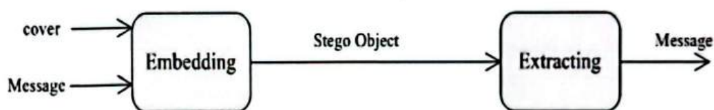
Fig. 3. Pure steganography process.
