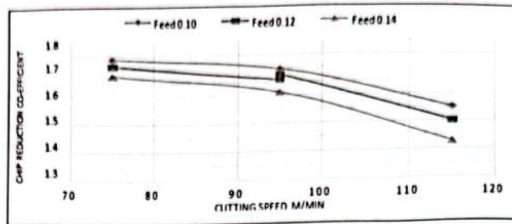
Fig 5: Chip reduction co-efficient vs cutting speed for different feed rate (room temperature)
